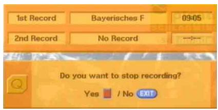
Using the screenshot above, you can also check the recording status without having to interrupt the recording. The stop time is indicated at the right of the top bar. Press to return to the full screen without stopping recording.
